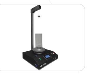
impact resistance including material thickness, uniformity of thickness, sample clamping, dart weight and drop height.
