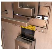
Two sample clamps above and below the Film Feeding Blade are used to hold the sample. In manual loading mode the user controls the clamps and loads a single sample. In automatic mode, the sample clamps are controlled by the PLC after initial loading on to a spool.
