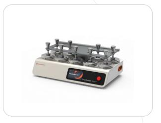
It can test the abrasion and pilling resistance of cotton, linen, silk woven fabrics and other textiles, film materials, knitted fabrics, woolen fabrics, artificial leather, synthetic leather, gloves, labor protection materials, and so on. It is widely applicable to more than 20 international standards such as ISO 12945-2-2020, ISO12947-2-2016, BS EN 530-2010; ASTM D4970/4970M-22, etc.
