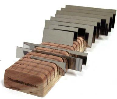
Test Panel Holder – Wooden holder with 24 angled slots to hold panels between tests. Dimensions: 12.5" (32cm) long x 3.5" (9cm) wide.
