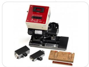
The SUTHERLAND® Ink Rub Tester performs five different tests: dry rub, wet rub, wet bleed or transfer, wet smear and functional rub.
