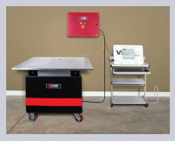
calculates the displacement with a known frequency and acceleration and then manually adjusts counter-weights on the vibration table to deliver the calculated displacement.
