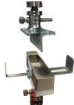
FLEXION TESTING FIXTURES (Corrugated Board) (3 and 4 Points of support) With fixed or variable support distances
