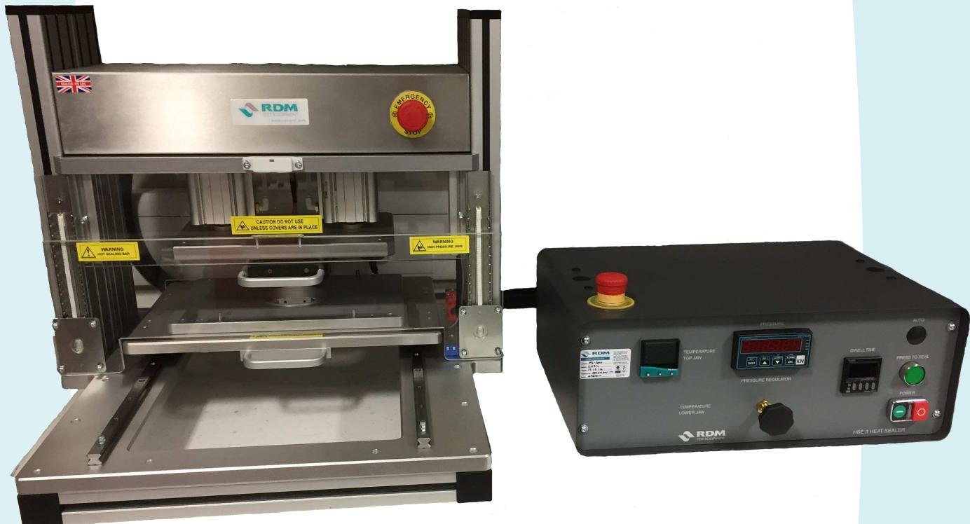
The HSP-2 Pot Heat Sealer is a customisable technology to deliver high quality heat seals for pot/lidding film packaging. A custom made pot holder and sealing platen are specified for individual sealed packs, or multiple seals across a pack.
