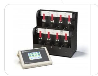
is compact and easy to use. It is also easy to read 0.5" (1 cm) LCD timer display is set to time in increments of 1/10 of a minute. Timer box operating temperature range 32° - 150° F (0° - 70° C). Timer box has universal input voltage from 85-265 VAC (50/60 Hz). Optional thermocouple accessory records failure temperature.
