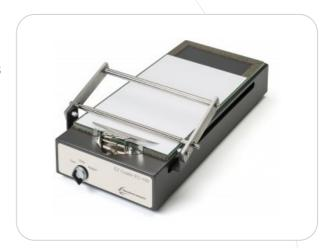
The Fixed Speed Drawdown Coater provides machine-controlled preparation of laboratory samples for adhesive, coating, ink and sealant testing. It's simple operation and lack of adjustments makes it the perfect shop floor tool to create consistent samples as well as greatly reducing the "human" interface for improved repeatability.
