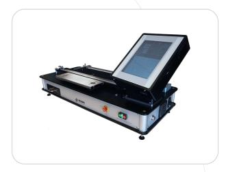
cartooning machine. Additionally, the instrument records the spring back force, which indicates the materials' resilience after the crease is folded. A great attribute for a carton tester as this can effect the way the carton behaves during the forming process and can also cause glued flaps to spring open before the adhesive has had time to cure.
